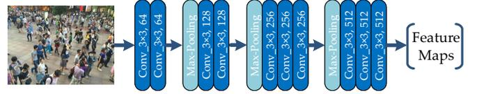
Fig. 3. **vgg-16 based encoder.** PSCC adopts vgg-16 as its image feature encoder, it only contains its first 10 layers, and discards these layers after the last max-pooling.
